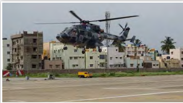
The first flight of Advanced Light Helicopter (ALH) – Wheeled Version with segmented Main Rotor Blades and Pre-Cone Main Rotar Head.
